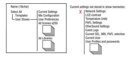
**Current Settings** Includes all the current mix parameters, processing parameters, preamp settings, names and colours, patching, effects, clock source, talkback and signal generator settings, and Surface strip assignments.
